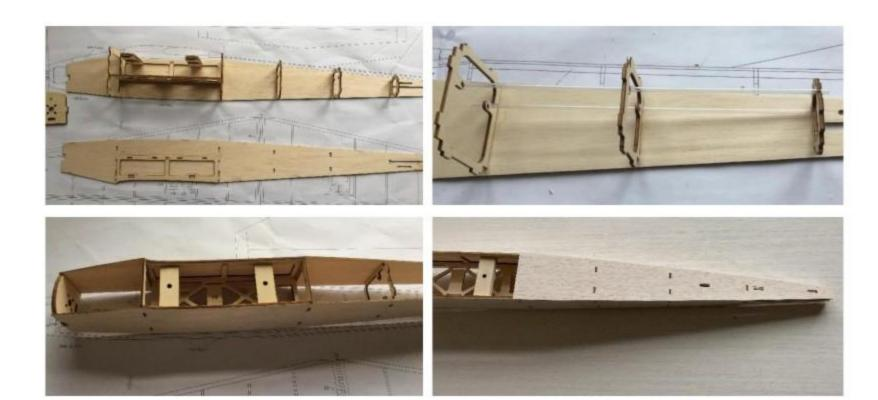
6. Paste 5MM balsa wood sheets to increase the strength of the head.
