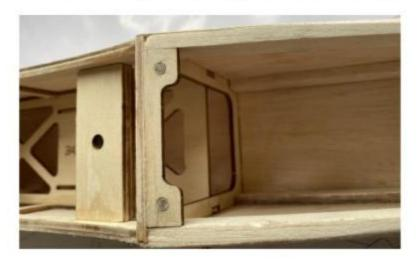
11. The leading end of hatch cover is fixed with a 1.6 mm steel wire bolt and pasted.
