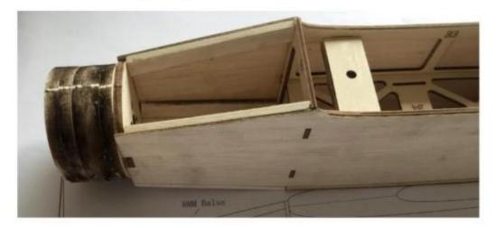
8. Make the battery hatch cover with 8MM balsa sheets.
