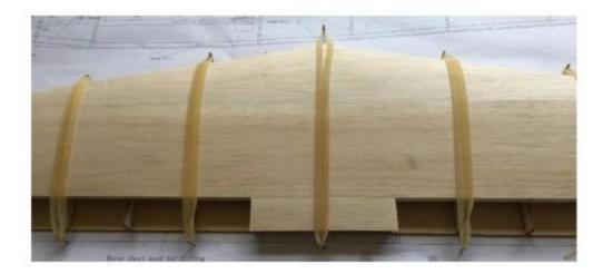
11.8MM balsa sticks were glued to the leading edge of the wing.
