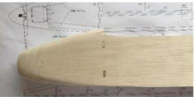
9. Mark the hatch cover at the corresponding position with the magnet fixing plate, drill a 4MM bit and fix the magnet to the hatch cover.
