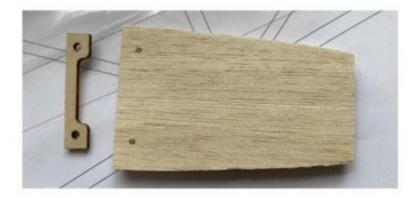
10.Install the magnet retaining plate into the fuselage.
