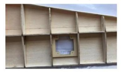
7. Paste the balsa stiffeners in the middle of the wing.
