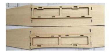
5. Combine and paste the parts according to the plan, and Install the PVC tube for pull-pull steel wires .
