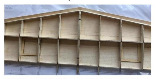
6.Cut out the opening at servos plate position and stick the servo stiffening plates.
