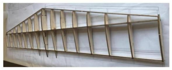
4. Paste the servo mounts to the wing ribs.
